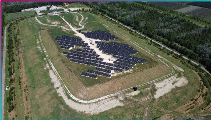
1 MW PV plant installed on an exhausted landfill started operation
